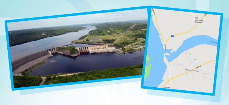
The Mactaquac Dam is an embankment dam used to generate hydroelectricity in Mactaquac, New Brunswick.
